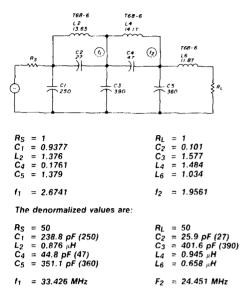
tune  $L_2$ .  $C_2$  for an attenuation peak at  $f_1$  tune  $L_4$ ,  $C_4$  for an attenuation peak at  $f_2$
